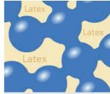
The mixtures is flash frozen to -30° Celsius, enabling the cells to retain their round form. The cell membranes break open and link together to create an open-cell structure.
