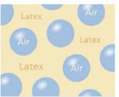
A precise mixture of natural and synthetic latex is mixed with air and stirred until an airy lather has been created, which is then poured into molds.
